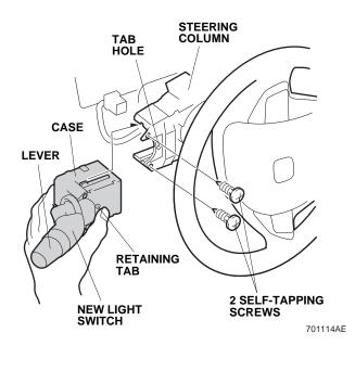
40. Plug the light switch connector into the new light switch. Make sure the vehicle harness is not being stretched.
