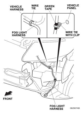
26. Secure the fog light harness to the vehicle harness with one wire tie.
