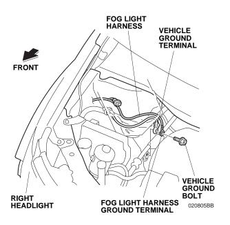
14. Locate the 1-pin connector blue-taped to the vehicle harness. Remove the blue-tape to release the 1-pin connector.
