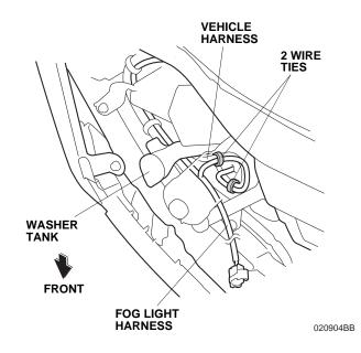
21. Route the fog light harness along the vehicle harness, and secure it to the vehicle harness with six wire ties.
