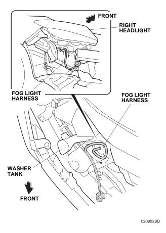
19. Secure the green tape on the fog light harness to the vehicle panel with one wire tie with clip.
